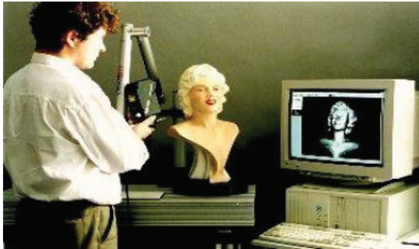
FIGURE II.1. Bras manuel et scanner 3D à bande (3D laser scanners: History, applications, and future)
