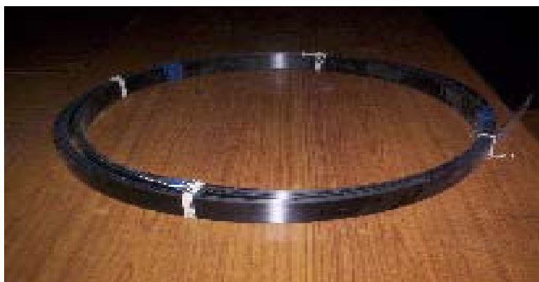
Figure 3-4 Lamelle sika carbodur.
