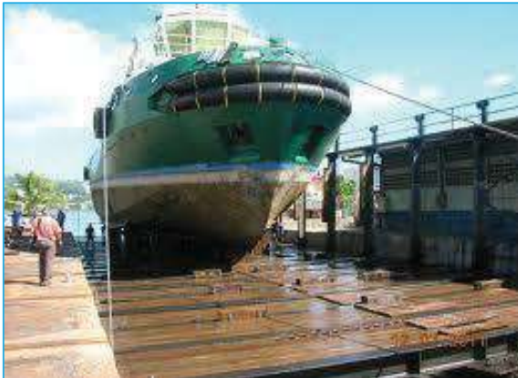
Figure II. 17: calle de hallage
