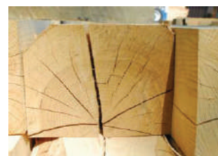
Figure I. 3 formations des fentes
