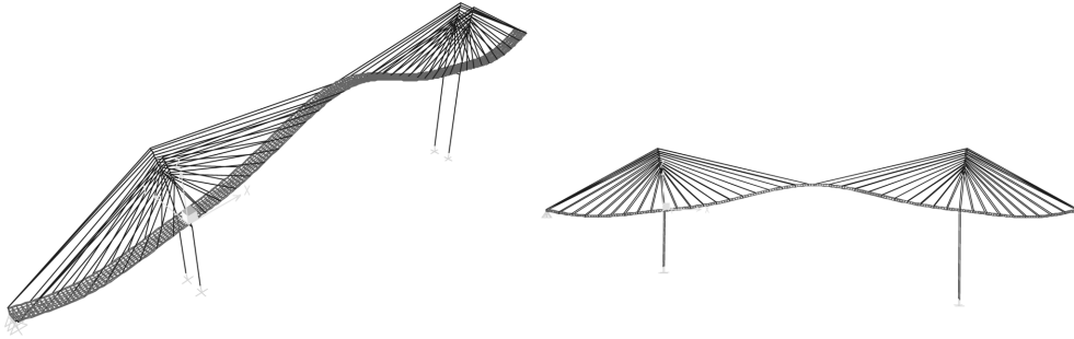
Fig. 4 First vertical bending mode at 0.34 Hz
