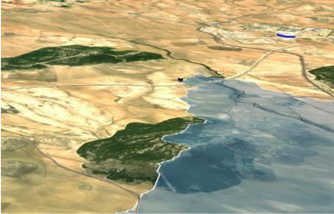
Figure I - 13 Automatic delimitation of a watershed by infraworks
