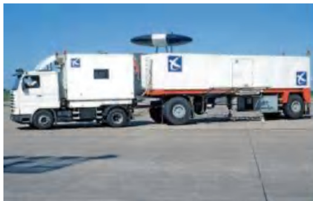
Figure III.5 Remorque de portance du STAC
