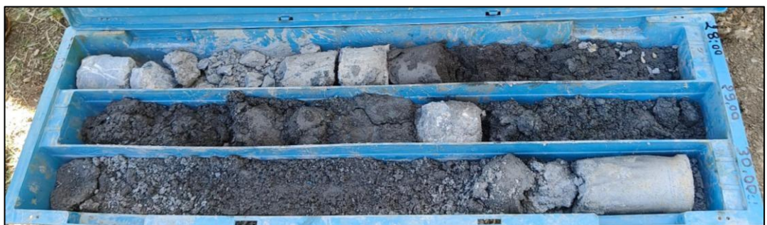
Forage/Borehole TBH-8, Caisse:9, 27.00-30.00 m
