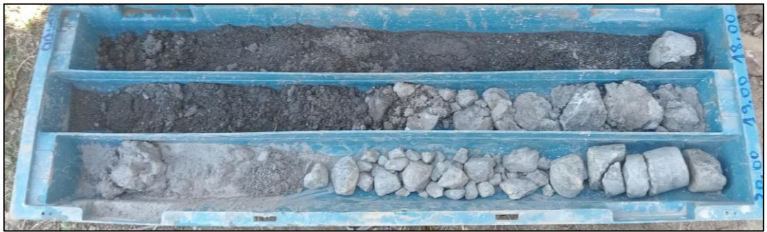
Forage/Borehole TBH-8, Caisse:6, 17.00-20.00 m
