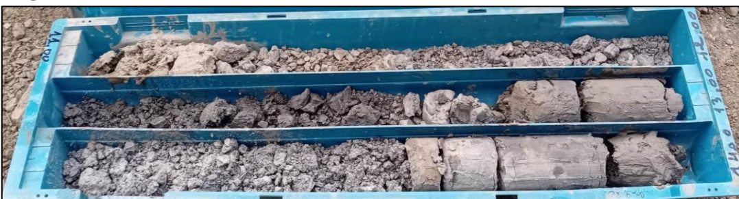
Forage/Borehole TBH-8A, Caisse:4, 11.00-14.00 m
