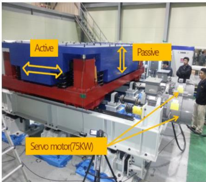
The components of Technomart Hybrid Mass Damper(HMD)
