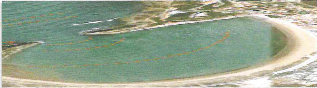
Figure II.14. Illustration de diffraction de la houle
