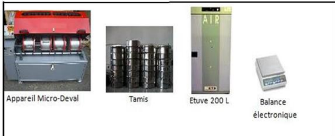
Figure II.5. Appareillage de l'essai Micro-Deval [17].
