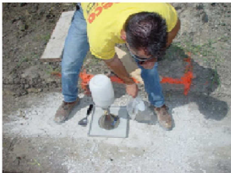
Figure V.02: Cône de sable (APWA; 2005)
