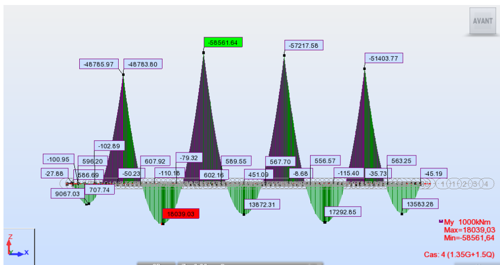
Figure II.18 Moment maximal Variante 3
