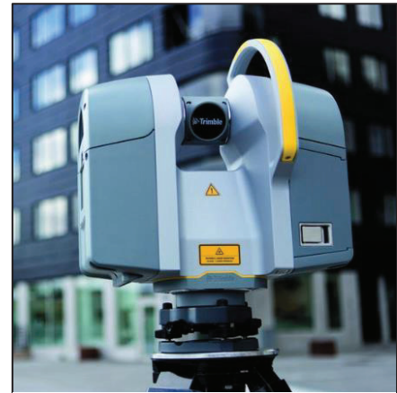
Figure I. 3 : Scanner laser 3D.
