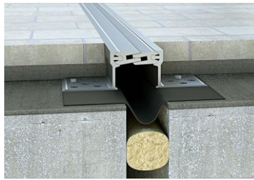
Figure I.2: Joint de dilatation. [5]
