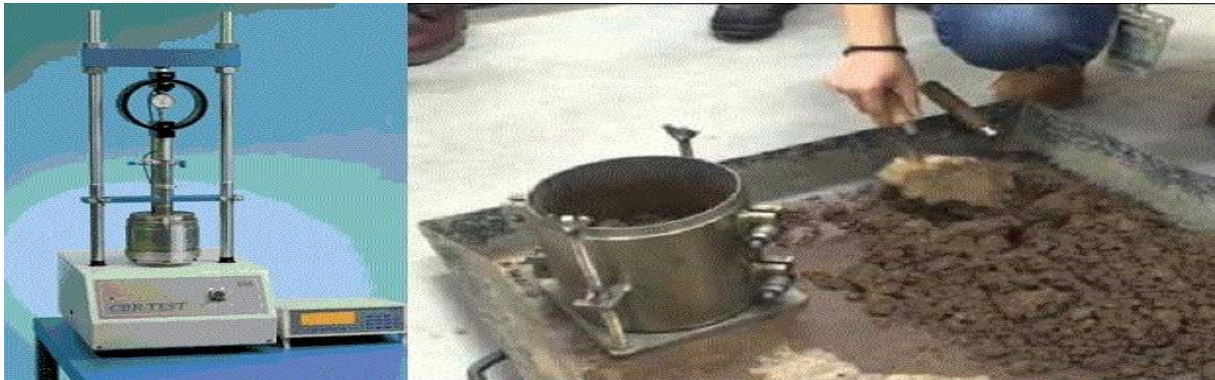
fig VI.7 Essai C.B.R (California Bearing Ratio)
