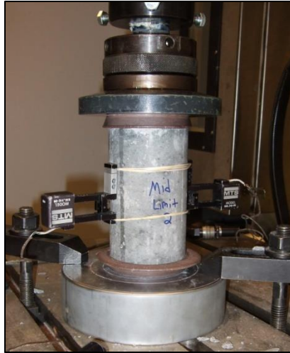
Figure 3: l'essai de compression simple.
