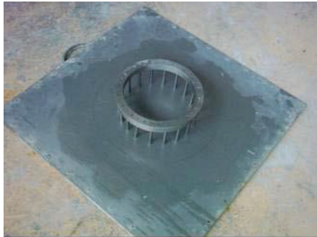
Figure III.13 : Essai de J-RING [41].
