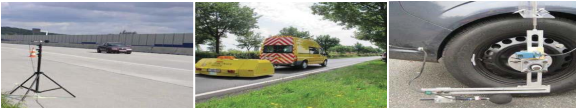
Figure I.2.4. SPB - Statistical Pass by Intensity, CPX - Close Proximity, OBSI - On Board Sound.
