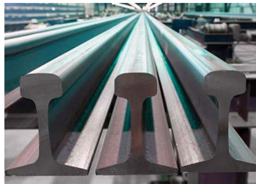
Figure II-1: Barre de rails UIC 60
