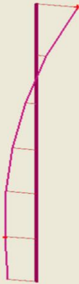
Horizontal displacements U_x
