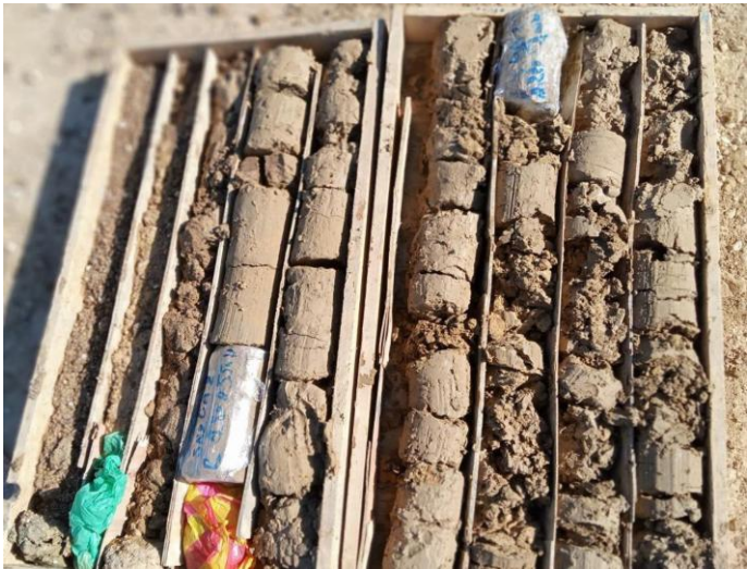
Figure A.2. SC1 cored borehole to a depth of 20 meters.
