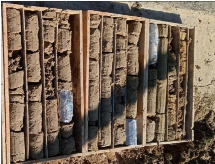
Figure A.4. cored borehole to a depth of 10 meters.
